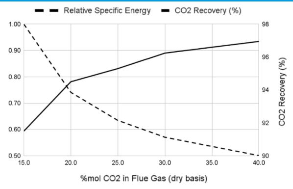
High purity CO2 feed to the liquefier results in less CO2 losses from the liquefier inert gas (N2/CH4/O2/CO) purge. Also (not shown on this diagram) dry CO2 to the liquefier results in less CO2 losses on the liquefier dryer unit. The holistic system CO2 losses, or CO2 capture rate must be analysed.
