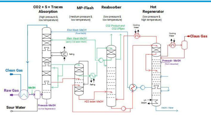
Linde (50 references globally) and Air Liquide / Lurgi (110 references globally) offer Rectisol™ using a chilled methanol solvent. The main energy input is compression energy for the methanol chiller circuit.
