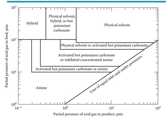
Chemical solvents (amine and HPC) react with the CO2 (chemisorption) and require high regeneration energies.
