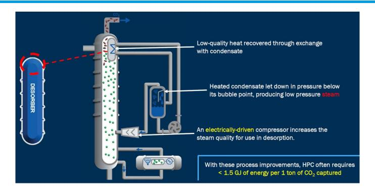
Full electrification: CapsolEoP™ claims 0.7 to 1.5 GJ Electrical power required per 1,000 tonnes of CO2 captured. The compressor / expander (compander) is key to operating the high pressure HPC process with a flash and recovering pressure energy from the flue gas.
