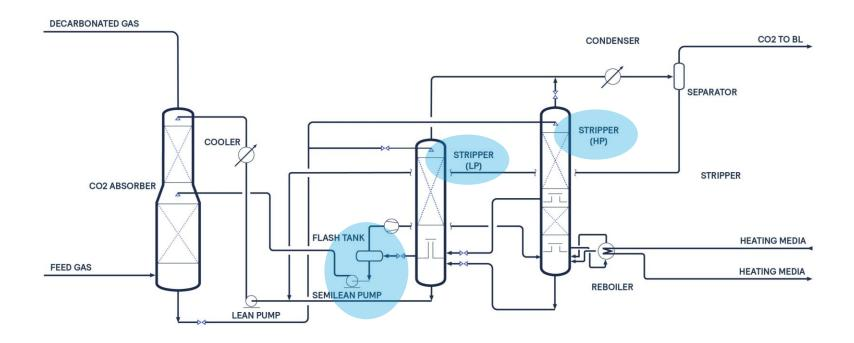
Baker Hughes chilled ammonia process (CAP). Previously developed by GE / Alstom. CAP has been demonstrated at various scales. It can either precipitate ammonium bicarbonate or operate fully in the liquid phase. Chilling reduces ammonia carry over with the flue gas vent. Energy demand is in the range 2 to 3 GJ/tonne CO2, like amines.
