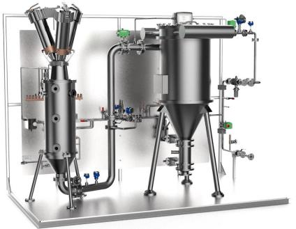
Levidian LOOP – microwave plasma methane pyrolysis, UK. Graphene production was the original goal and remains a key aspect of the business case for deployment.
