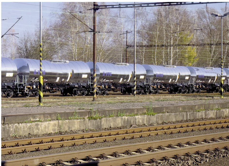
Bulk liquid movement by rail – a cement plant capturing 1 MT CO2 per year would need one train per day with 30 waggons to transport liquefied CO2
